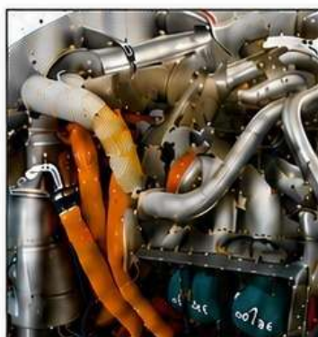
High Temperature Exhaust Lines
